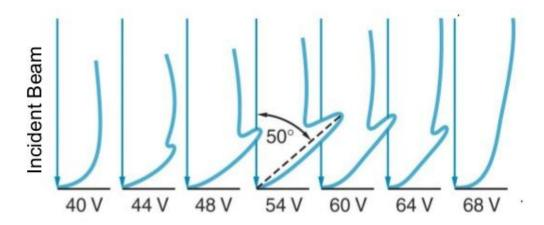
Current vs accelerating voltage has a maximum (a bump or kink noticed in the graph), i.e. the highest number of electrons is scattered in a specific direction.
